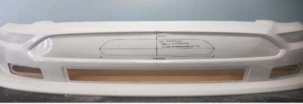
**ANNEXURE 17:** Full wear strip attached to One-piece fibreglass nose assembly.
